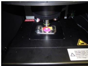
Micro-SORS analysis of three layers system at CNR-ICVBC, Milan
